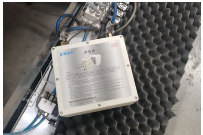
Silencers were installed to vacuum sound-emitting components
